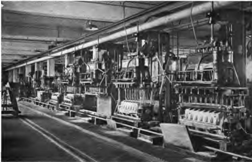
**Section of Track System for Machining Upper Half of Liberty Motor Crank Case, Lincoln Motor Co.**
